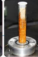
Optionally the system can be equipped with tube sample holders. A supplied set has four replaceable tube holders with plastic lids, which can be attached to a sealed baseplate. The tubes are 8 cm high, with internal diameters of (approx.) 6, 10, 15, 20 mm. The tube holders allow scanning samples with different sizes, including automated batch scanning, and imaging of hydrated samples and samples in liquid.
