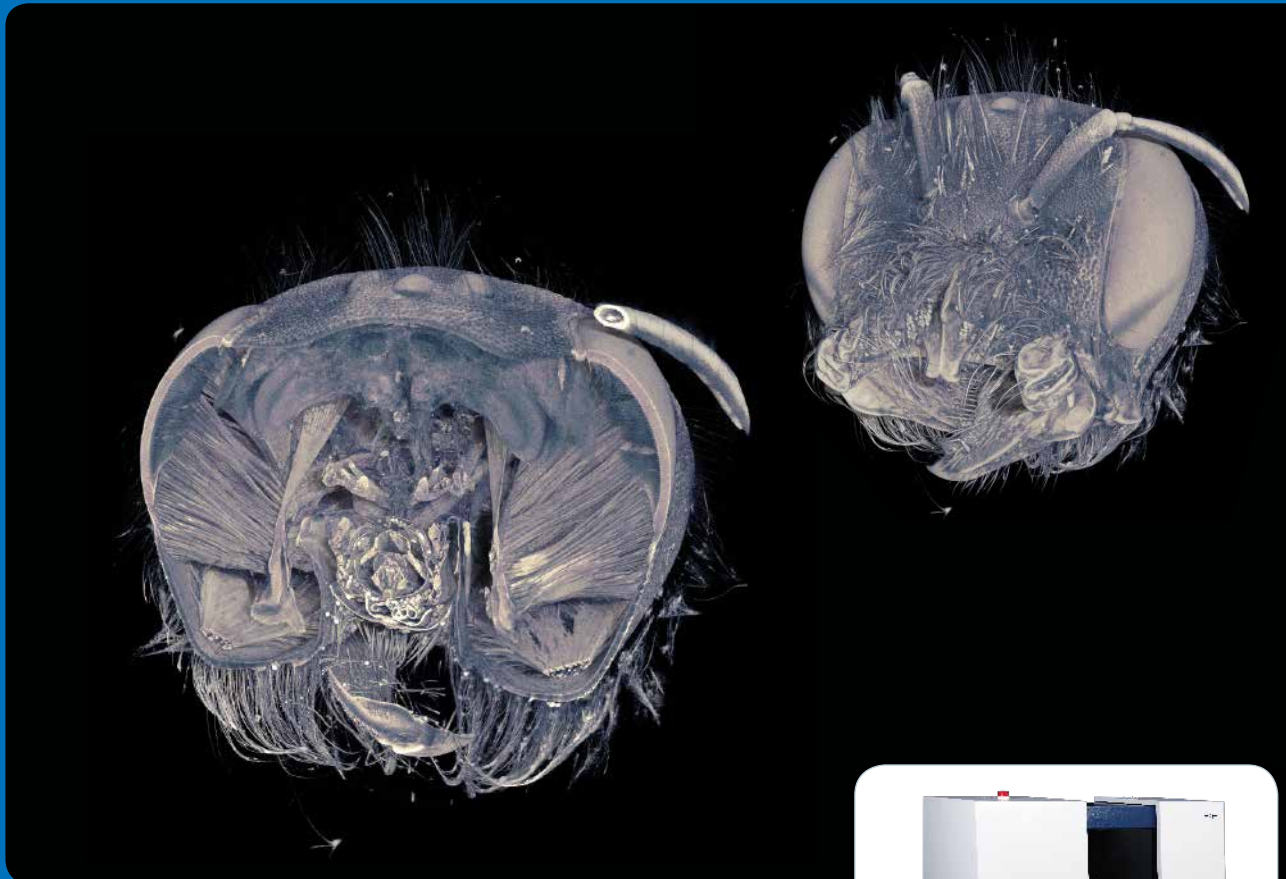
Volume rendered 3D model of a mason bee head, scanned at 1.4 \mu\text{m} pixel size (collaboration with Prof. Javier Alba-Tercedor, University of Granada, Spain).
