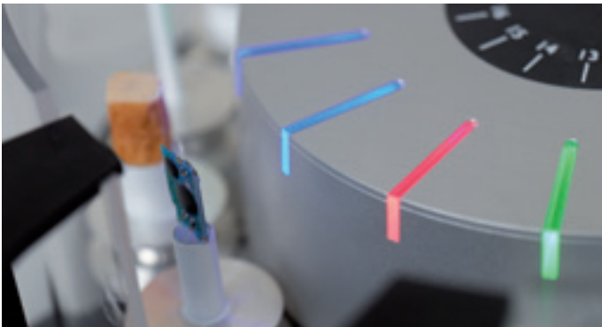
Autodetection of new samples and status LEDs for every scan: ready, running, done
