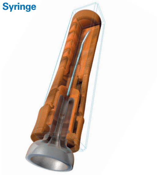
Non-destructive analysis of a syringe needle SKYSCAN 1275 – Voxel size 10 \mu\text{m}
